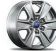
18" Silver Heavy-Duty Aluminum XL – Optional: requires 101A and Heavy-Duty Payload Package XLT – Included: Heavy-Duty Payload Package LARIAT – Included: Heavy-Duty Payload Package
